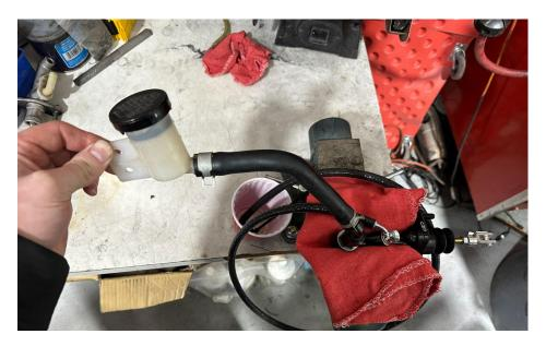
22. Making sure to go underneath the two ABS lines, run the clutch line through the grommet at the front left hand side of the brake cubby (from which we removed the old hard line) and route it along the inner fender skin, following the routing of the stock line.
