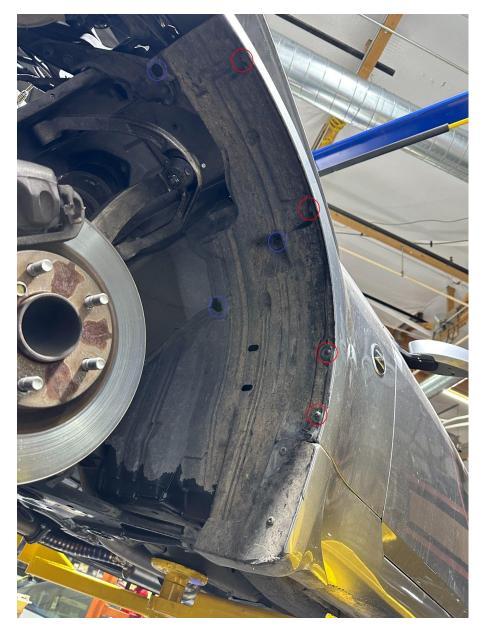
13. Start with the four phillips screws going along the edge and bottom of the fender. Then for the remaining clips, remove them in the same way as performed earlier with the pop clips for the brake cubby surround. Once all seven of the plastic pop clips have been removed the rear half of the fender liner should come right off revealing the clutch hardline. For people whose cars have the OEM mud guards, you will have to remove those as well.
