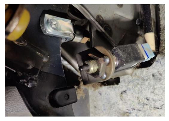
31. After checking for any leaks or loose hardware in the cubby, go ahead and reinstall the brake cubby cover with the five plastic clips we removed in step 5. You can also fit the lid for the cubby now.
