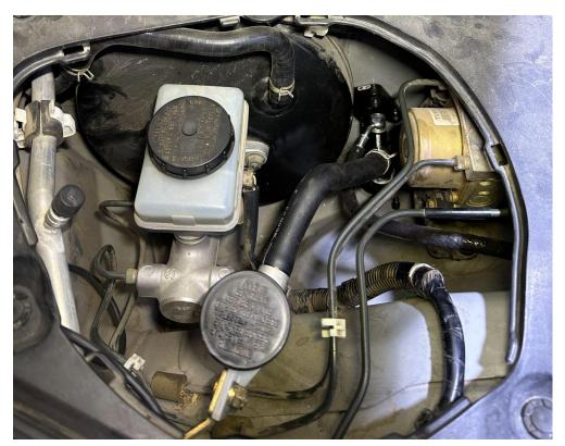
27. Grab the loose 90 degree end of the clutch line we fed through the grommet to the fender well earlier. This end goes under the chassis rail behind the compression rod to the stock clutch line bracket that is on the chassis, next to the transmission and the short clutch leader line we unscrewed the stock hardline from earlier. Screw the fitting into the line that is clipped to the chassis and tighten it down with a flare wrench. (Torque spec for the union is 11-12 lb-ft or 15-17 N-m)
