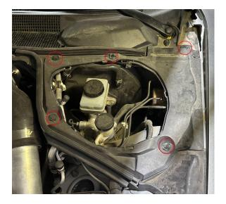
6. Unbolt the flare nut for the high pressure line (circled in blue) from the master cylinder using a 10mm flare nut wrench.
