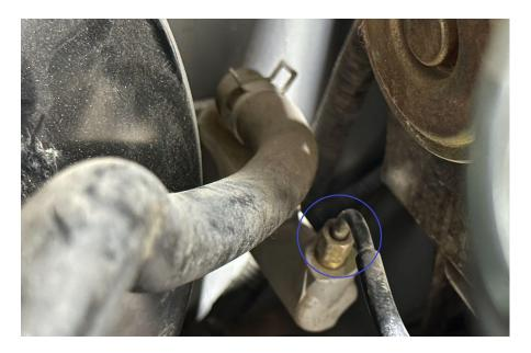
7. Remove the two 10mm hex M6 nuts and their washers (circled in red) that are holding the clutch master cylinder reservoir to its bracket but leave it connected to the master as we will be removing it at the same time, as one complete unit.
