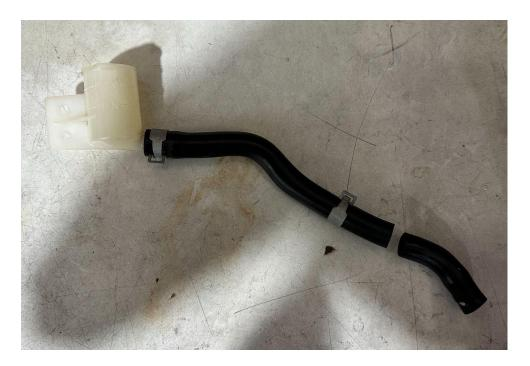
21. Install the reservoir hose onto the wilwood master and secure it with the stock spring clamp.
